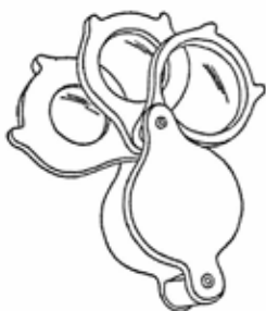
A magnifying glass having three lens that will magnify from five to twenty times
